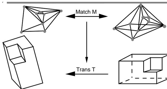
fig 4.1: the "matching" process: left the scene object and its PFRG, right the reference object and its PFRG
