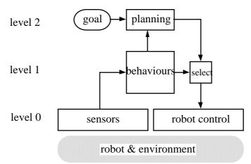
Fig. 1 Principe of the behavioural mobile robot navigation system
