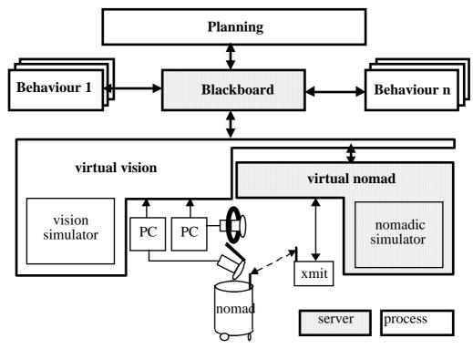
Fig. 7 Architecture and unix processes
