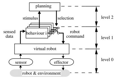
Fig. 4 Control structure of MANO
