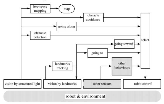
Fig. 2 Vision-based behaviours
