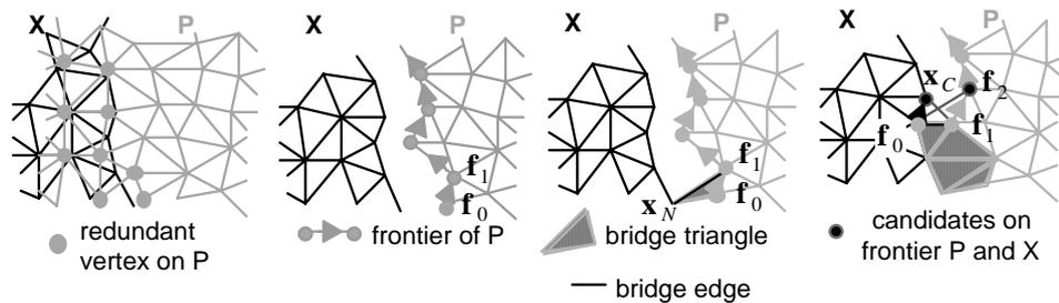
Fig. 4. Mesh fusion showed for an example
