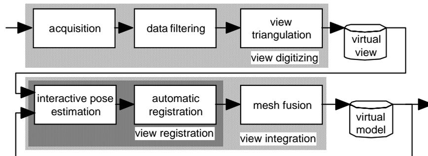
**Fig. 1.** Digitizing system architecture
