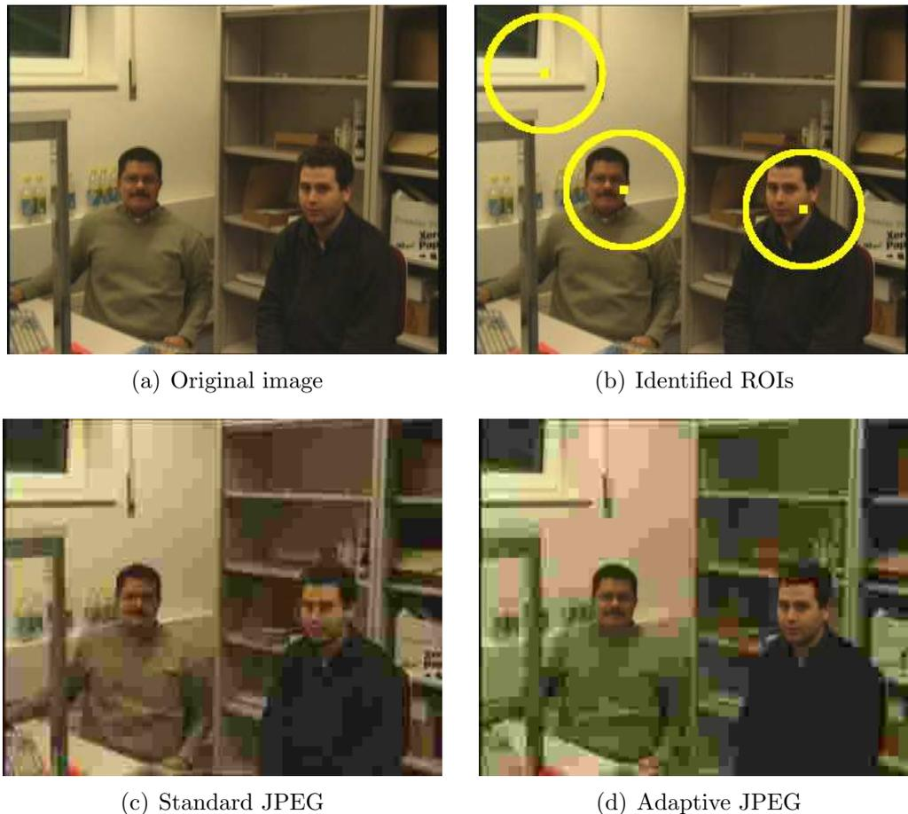
Figure 6.4: Adaptive versus standard JPEG: Example 1.
